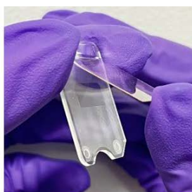
(b) Open Q-Card by lifting the thin film of the top plate at the notch.
