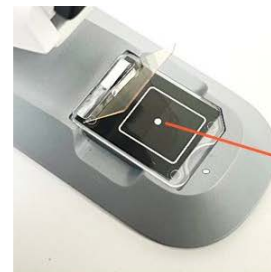
(d) Put Q-Card on and secure it in the "Card Slot" of Presser.
